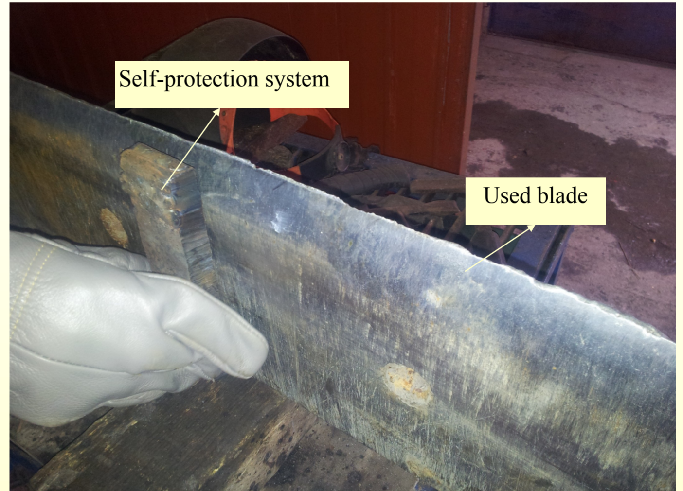
Pushing blade with wear and self-protection system
