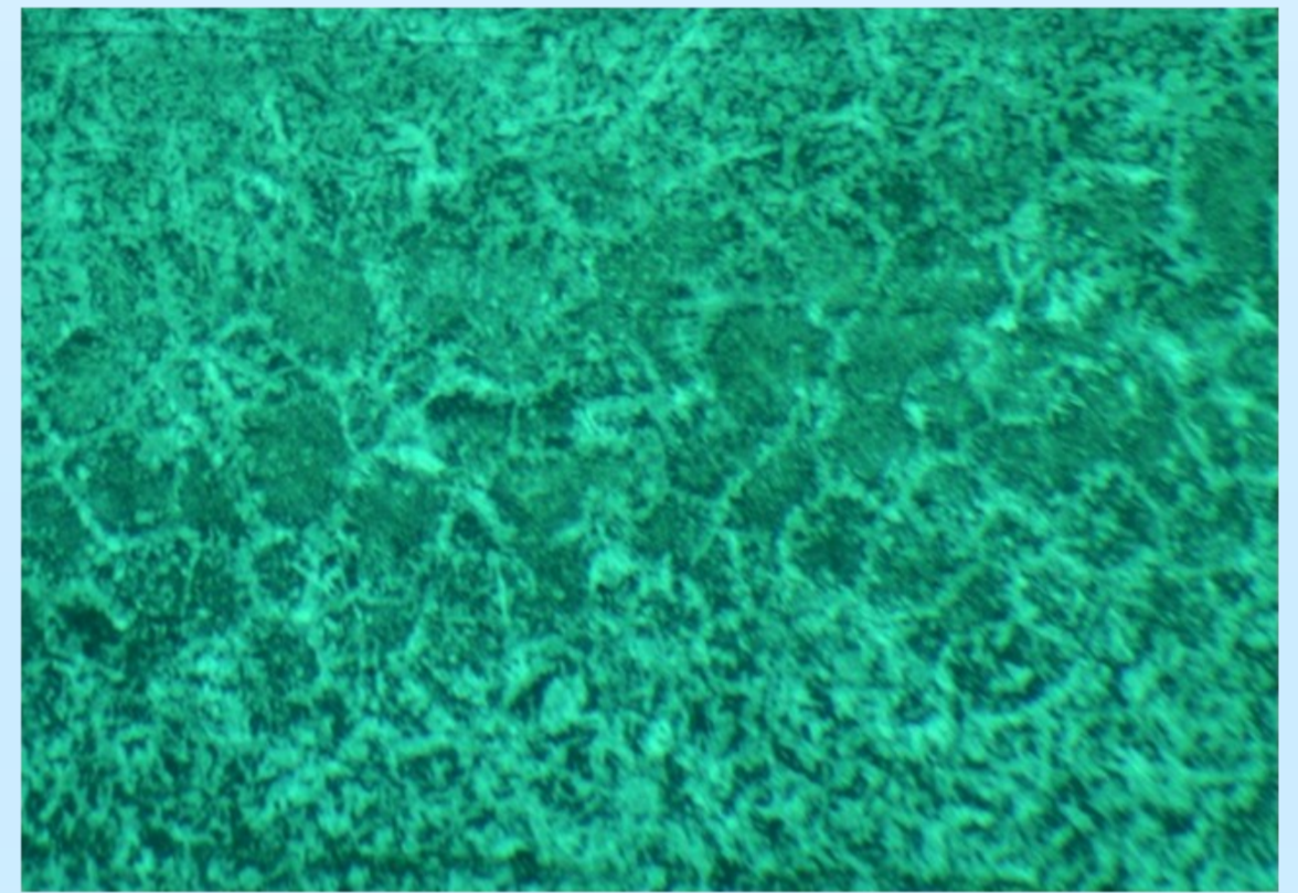
Deposited metal. Fine casting structure [ 100X]
